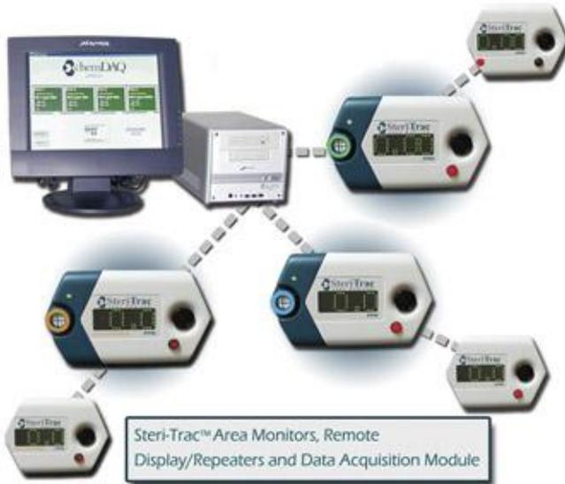
The DAQ can operate up to four zones, each with up to 8 monitors, thus a single DAQ can be connected to up to 32 different monitors of any gas combination offered by ChemDAQ.
